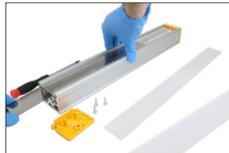
Insert the polarizer under the TR window
