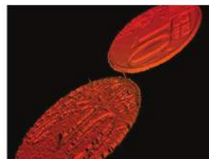
3D projector EFFILUX (on top) VS Laser (below) : no speckle so more accurate
