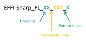
Near Field: NF for WD=[40;70]mm Middle Field: MF for WD=[70;150]mm Far Field: FF for WD=150;350]mm
