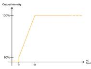
By adjusting the analog tension, light intensity can be controlled from 10% to 100%. If the Input AIC is not connected, the ELL will act as if AIC was set at 24V.
